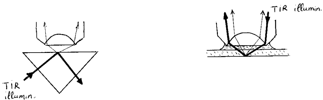
Figure 2.10 : Illumination of a sample by total internal reflection, either with a high-index prism in the case of a low index sample (left), or via the objective lens itself in the case of a sample close to an interface to a lower index (air or water, right).
