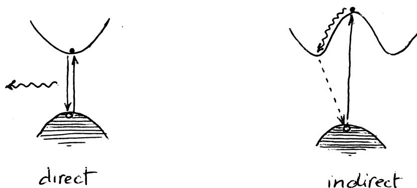
Figure 14.1: Energy-wavevector diagram (dispersion curve) for direct and indirect semiconductors. Because the wavelength of light is large, optical transitions are nearly vertical in the diagram, and are therefore forbidden for the relaxed state in indirect gap semiconductors such as Si and Ge.
